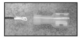
When crimping the temp. probe, strip back the insulation, then fold wire back on itself to double thickness.
